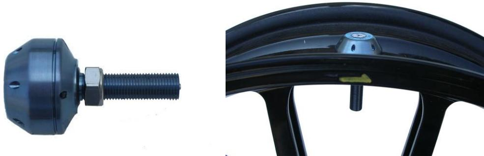
Measures and transmits tyre pressure and temperature, provides continuous monitoring of motorcycle tyres during test, practice and race conditions. Operates with TMS AS Receiver. Installs in a standard 8.8mm valve hole with O-ring seal as a valve replacement, accepts standard valve core. All valve threads conform to ISO 4570:2002
